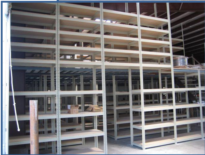
Shelving on both Levels for High Density Storage w/Catwalk Flooring
