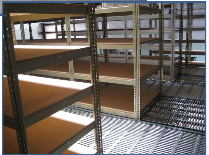
Shelving on both Levels for High Density Storage w/Catwalk Flooring
