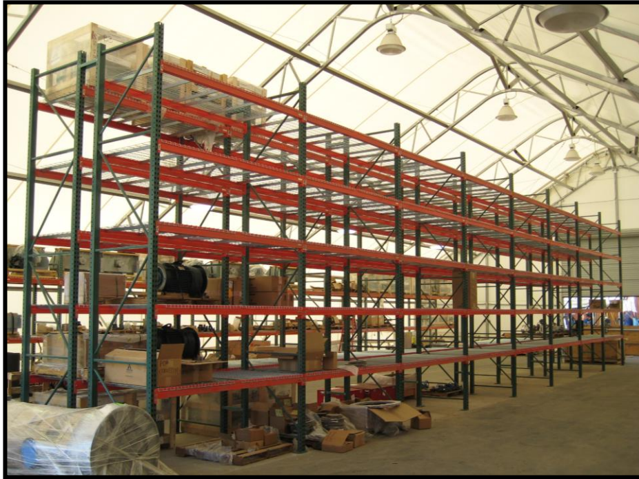
Pallet Racking: 5 Levels
