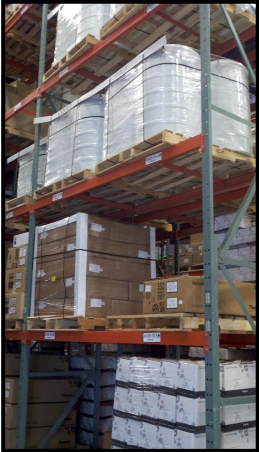
25' Tall Structural Pallet Racking 350 Pallet Positions | 42' Safety Rail
