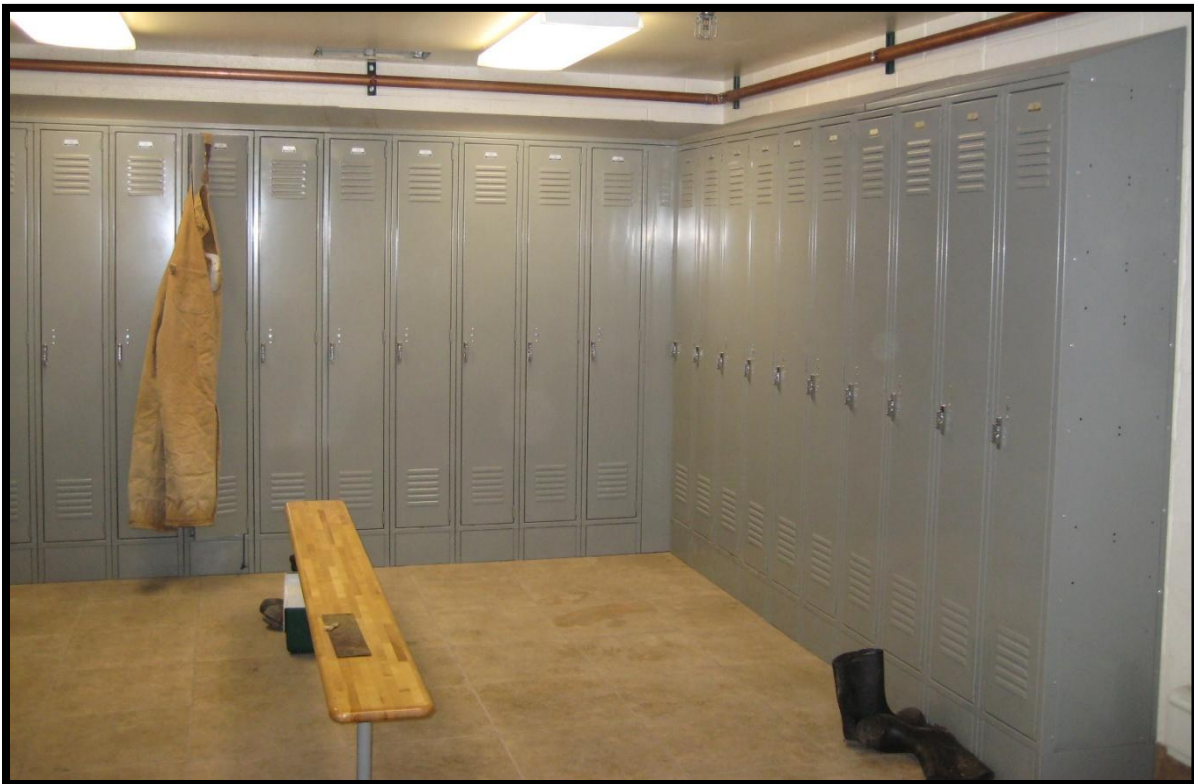
Single Tier Metal Lockers with Sloped Tops and Bases Locker Room Benches with Maple Tops and Metal Bases
