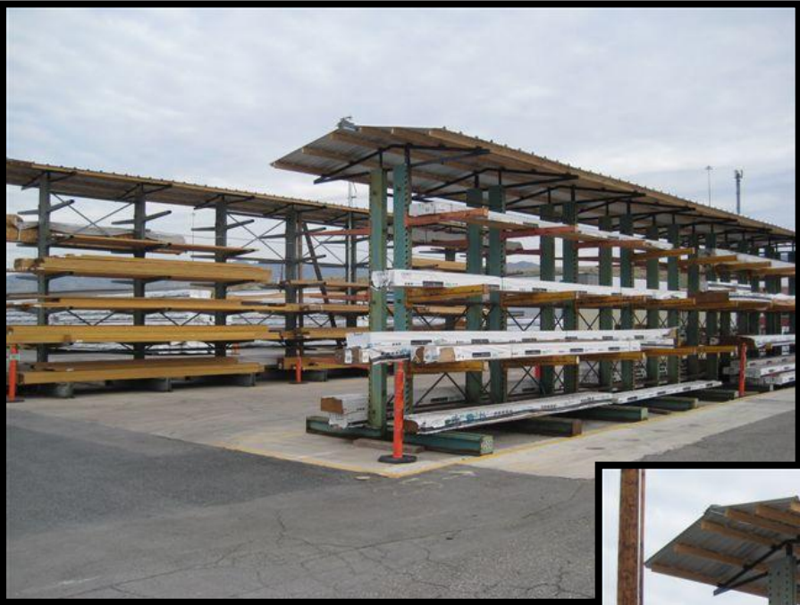
Custom Built Roof Supports that Utilized the Height of the Uprights
